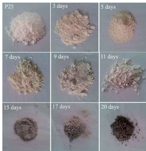
Fig. 2-1. Photos of P25 treated under H_2 for 0-20 days at 35 bar H_2 and room temperature.
