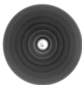
Fig 1-8 Typical detector output confirming the wave nature of the electrons.
