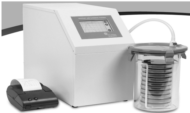
Fig. 2: Anaerobic gas jar system used to create an anaerobic and microaerophilic environment in Gas-Jar.
