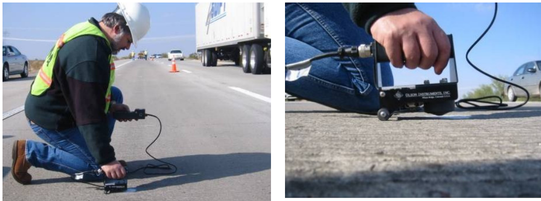
Figure 1-21 Void detection in concrete by using IE method [112]
