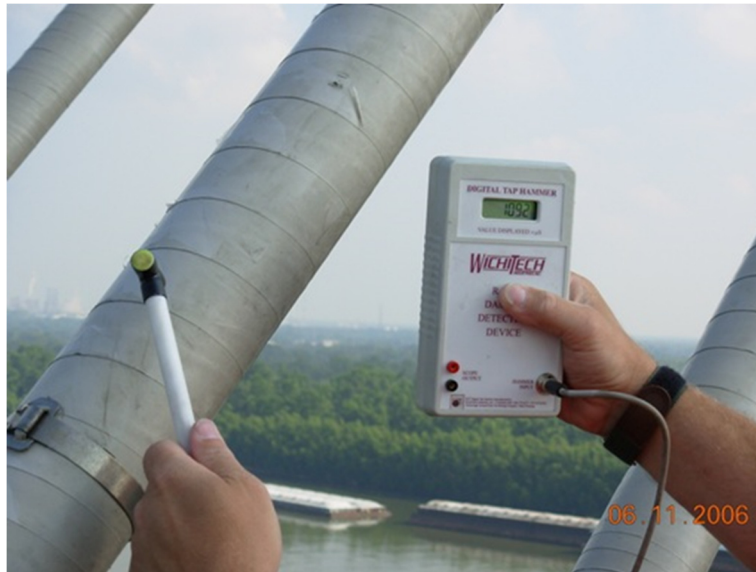
Figure 1-8 Use of digital tap tester for inspection of stay cable
