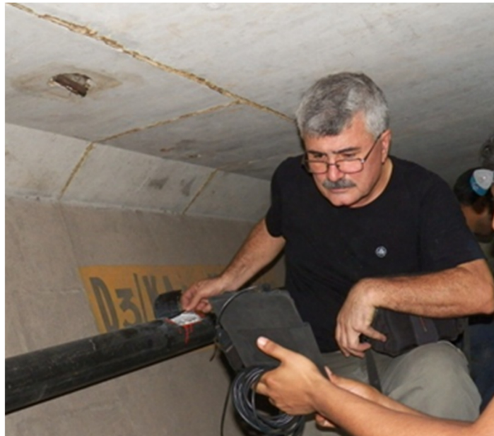
Figure 1-3 Use of borescope for inspection of voids in PT ducts
