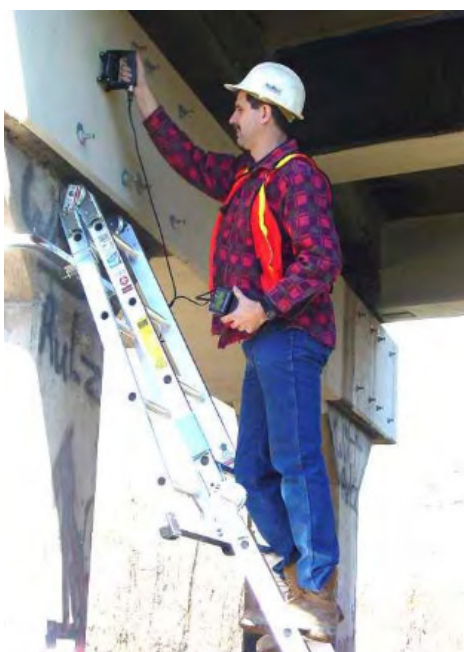
C. Impact echo measurements
