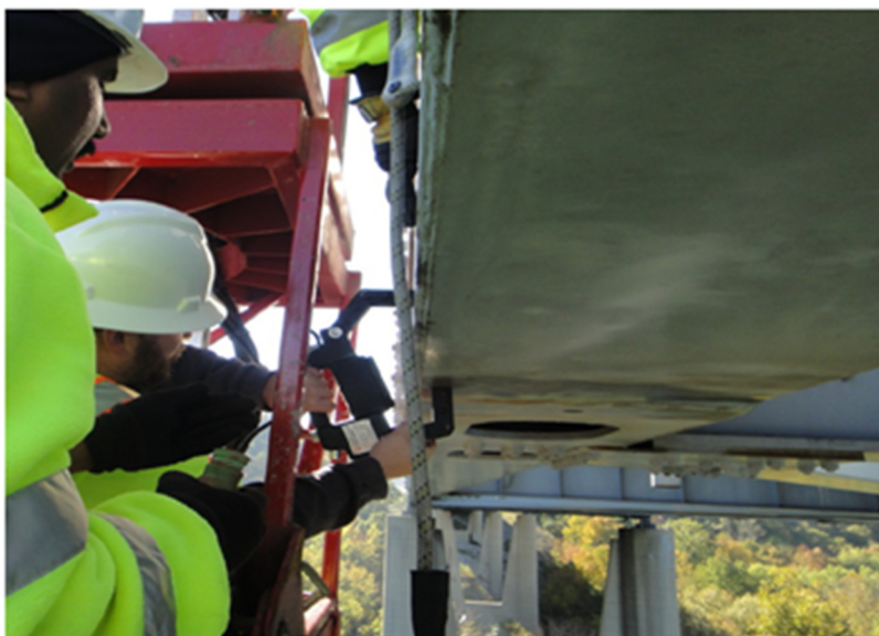
Figure 1-5 An example of MT inspection [3]
