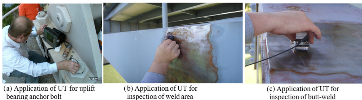
Figure 1-10 Applications of UT for steel bridges [3]
