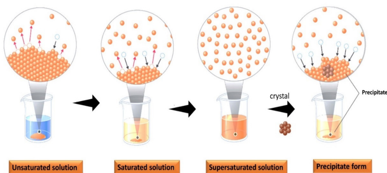
Figure 1.1 Schematic representation of Dissolution and Precipitation
