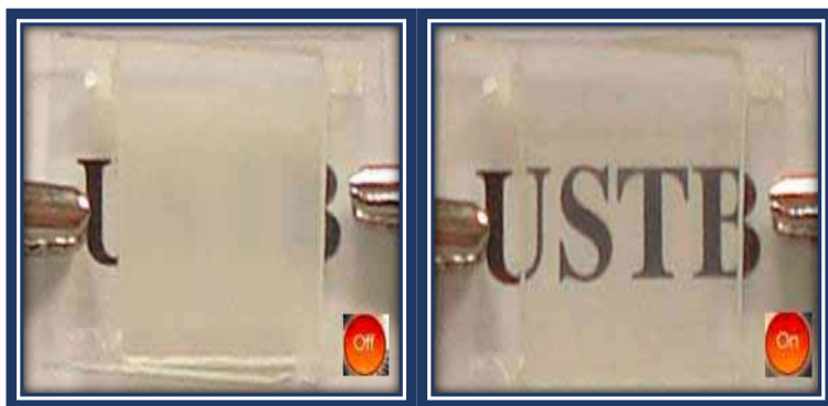
Figure 1-3 Schematic drawing of the PDLC film electro-optical application
