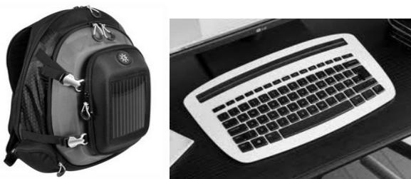
Figure 2.5: Two examples of DSC products: a solar backpack (left) and a wireless keyboard (right). [52]
