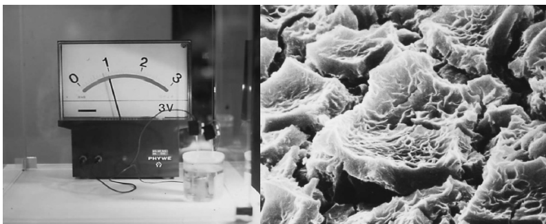
Figure 2.2: Left: the first DSC embodiment (1988). Right: SEM picture of the \text{TiO}_2 film used in the first DSC. Image adapted from [19].
