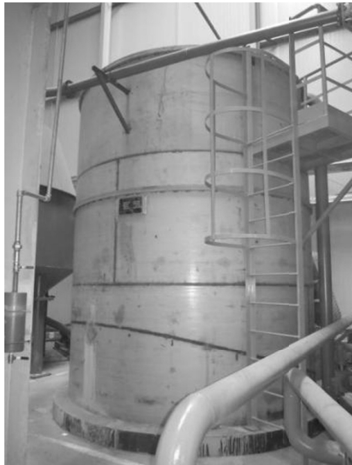
Fig. 1-12. Sample buffer pulp tank with a capacity of 30 m 3 .
