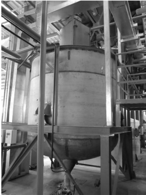
Fig. 1-16. Liquid mix buffer tank with a capacity of 11 \text{ m}^3 .
