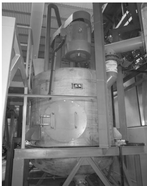
Fig. 1-15. Mixer with a capacity of 4.6 \text{ m}^3 .
