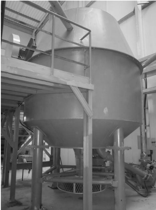
Fig. 1-11. Sample pulper with a capacity of 14 m 3 .
