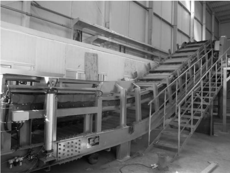
Fig. 1-9. Sample belt conveyor with scales (weighing cellulose and waste paper) feeding weighed-out portions into the pulper.
