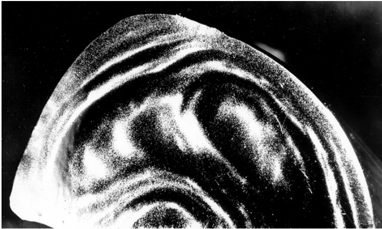
Fig. 1.3. Swirl distribution of B-microdefects in the plane [111], selective etching, crystal diameter 30 mm
