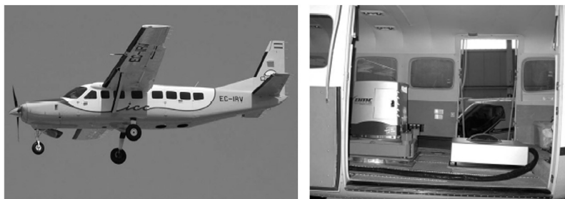
Figure 1. The ICGC aircraft used with the lidar installed on board (photo from www.icgc.cat )
