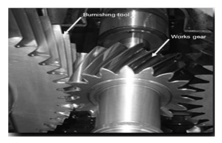
Fig. 1.8: Illustration of gear burnishing process.
