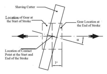
Fig. 1.7: Schematic of transverse gear shaving process.
