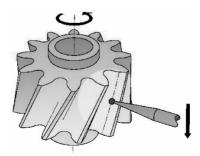
Fig. 1.3: Concept of measurement of lead error of a gear.
