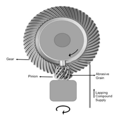
Fig. 1.10: Schematic of gear lapping process.
