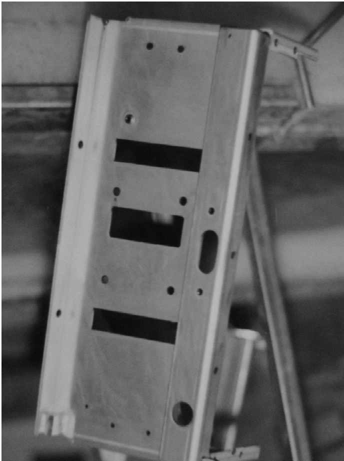
Figure 2.1: Aluminum surface cleaned too strongly and then conversion coated.
