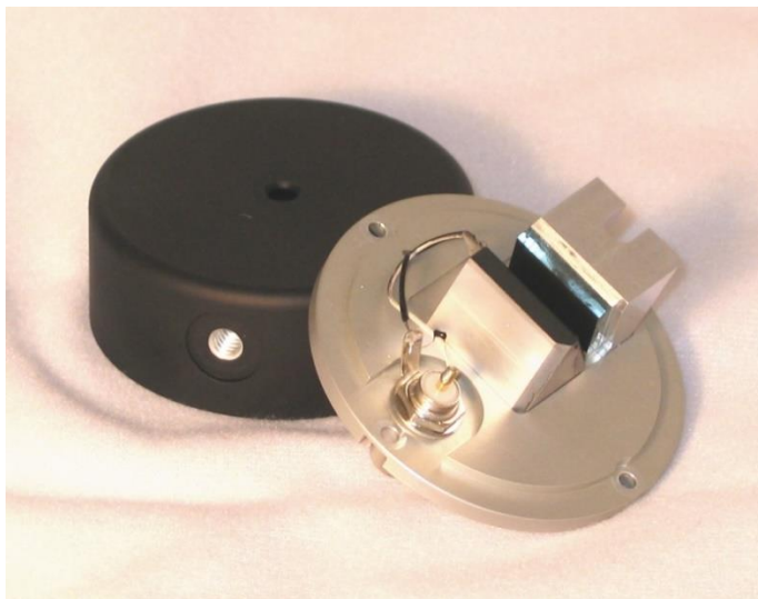
Fig. 11. Picture of the wedge-input pyroelectric detector shown in Fig. 10.
