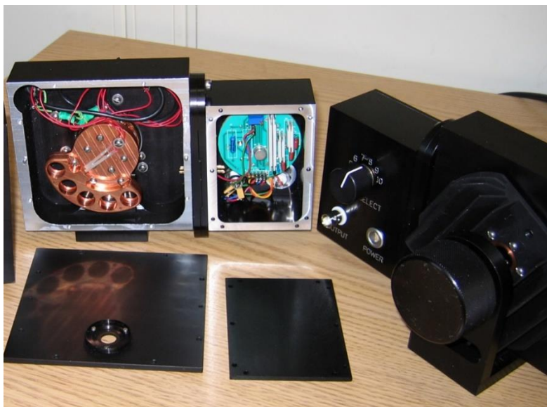
Fig. 2. Front and back pictures of two (single-element Si photodiode used) transfer-standard photo/colorimeters.
