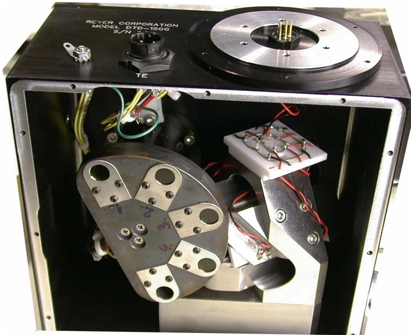
Fig. 1. Filtered trap-detector based transfer standard photometer.
